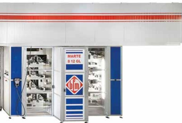
ket change in the machine. The sleeve system for quick change, in the machine, for both plates and anilox, nowadays a must in our market, has a pneumatic ejection to make it even easier. It is also possible the ejection of the plate sleeve in printing position, for the cliché cleaning.
